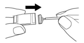
Figure 4-19 Disconnecting Bluetooth cable
